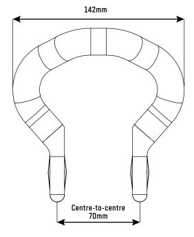
We recommend that a minimum of 70mm is available for clamping around a 31.8mm diameter length.
